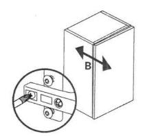
B-LATERAL Loosen screw 'B'. Adjust door and re-tighten screw.
